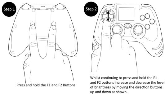
When setting the level of brightness whilst you are not within the TurboFire EVO menu, the lowest level of brightness will set the display panel to off. The display panel will remain off until you re-enter the TurboFire EVO Menu or increase the level of brightness.
